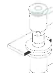
Fig. 4 Measurement of flat material (e.g. foamed material) with flat measuring contacts without tipping or sliding the gauge.
